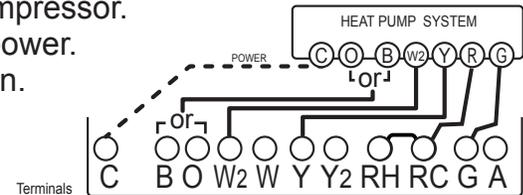
**Wires** **C W2 W Y Y2 RH G** **2 Stage Heat and 2 stage Cool**
