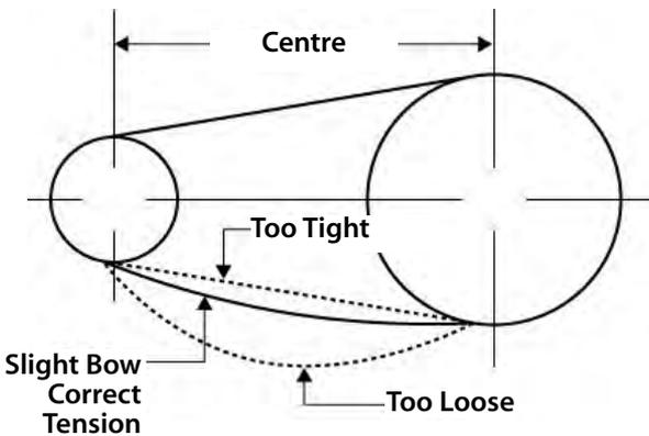
If the belt is installed too tight, the motor might be overloaded. This will cause the motor to overheat. If the belt is installed too loosely, it will slip and excessive wear and vibration will occur.
