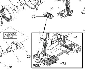
As an aid for servicing, the Speed Switch Assembly #72 should be mounted onto the PCBA first and than carefully installed together into the Left Housing Halve #1.
