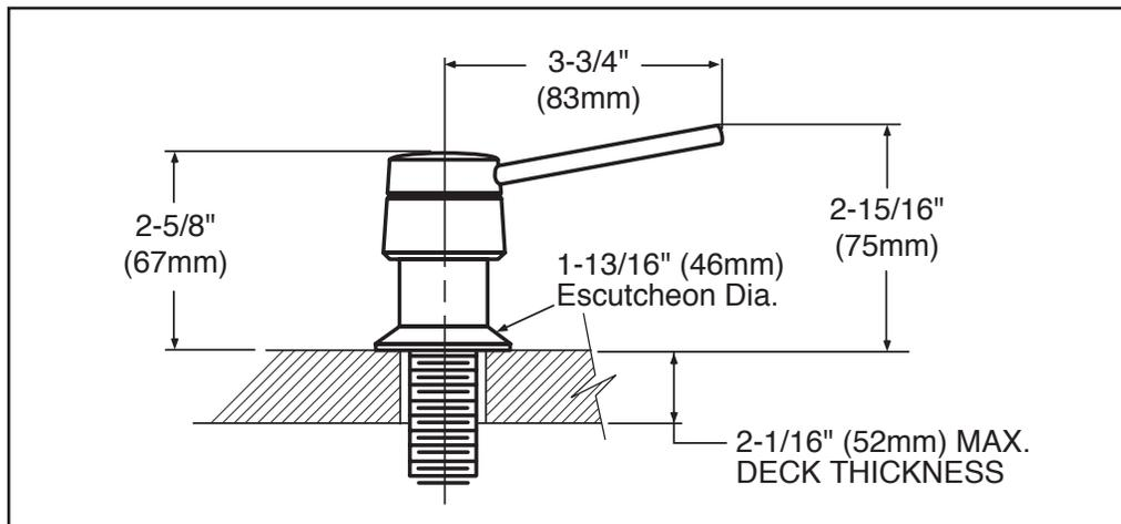
**NOTE:** DESIGNED TO BE INSTALLED THROUGH 1
