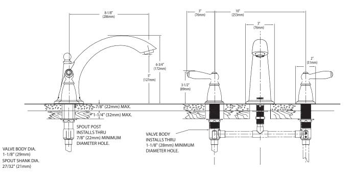
NOTE: THE INSTALLATION SHOWN IS FOR TILE DECKS, THIS VALVE WILL ALSO FIT STEEL. CAST IRON OR PLASTIC DECKS
