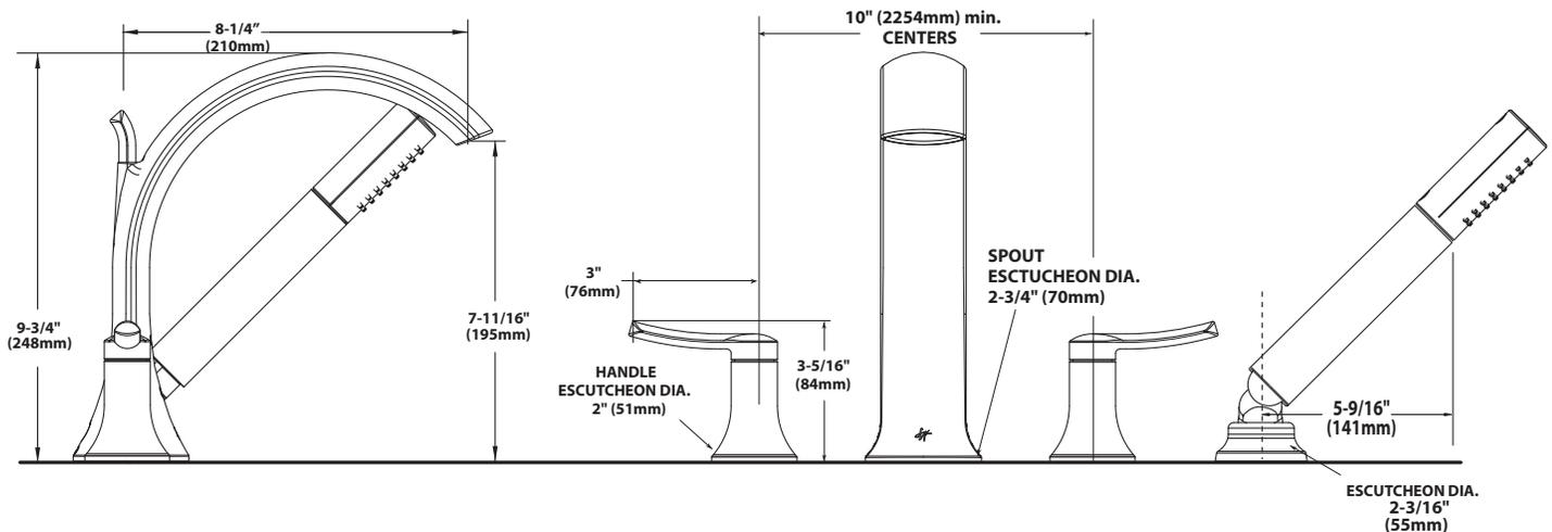
**NOTE:** THE INSTALLATION SHOWN IS FOR TILE DECKS, THIS VALVE WILL ALSO FIT STEEL, CAST IRON OR PLASTIC DECKS
