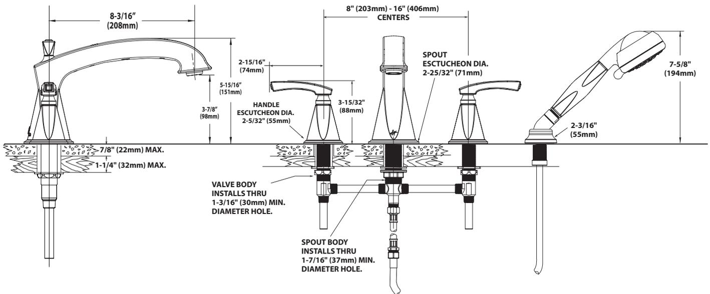
**NOTE:** THE INSTALLATION SHOWN IS FOR TILE DECKS, THIS VALVE WILL ALSO FIT STEEL, CAST IRON OR PLASTIC DECKS
