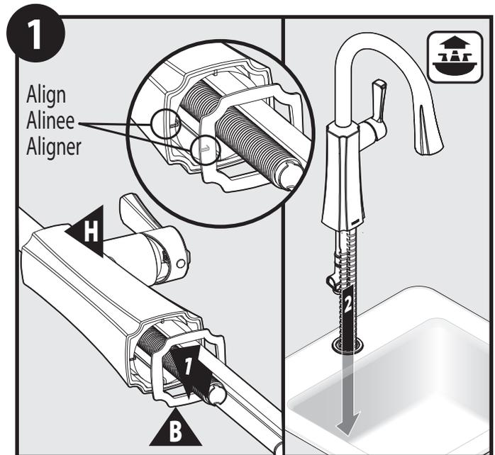
Place deck gasket (B) onto base of faucet body (H). Place into sink hole. **NOTE:** Install with handle on right side only.
