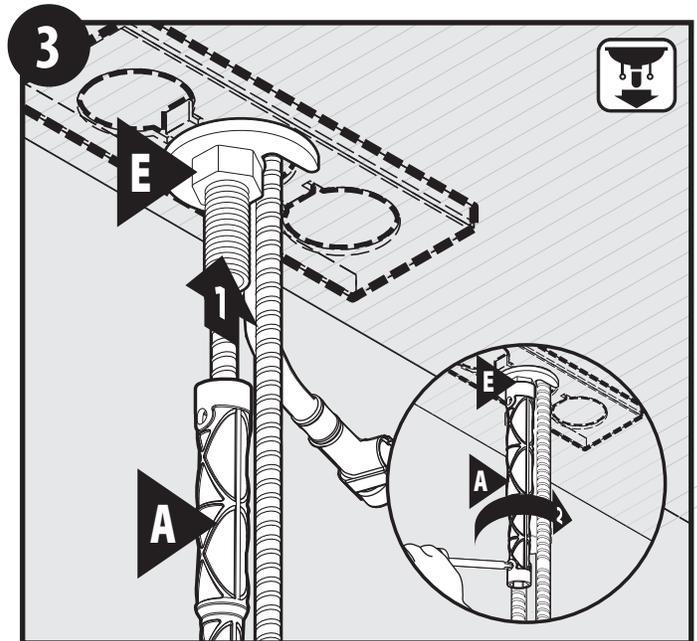
Tighten mounting nut (E) with installation tool (A). Use screwdriver through hole in installation tool (A) to tighten firmly.
