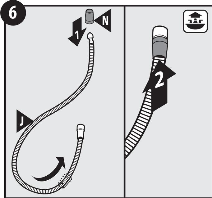
Slide hose swivel cover (N) onto pull-down hose (J). Push over swivel until cover snaps in place.
