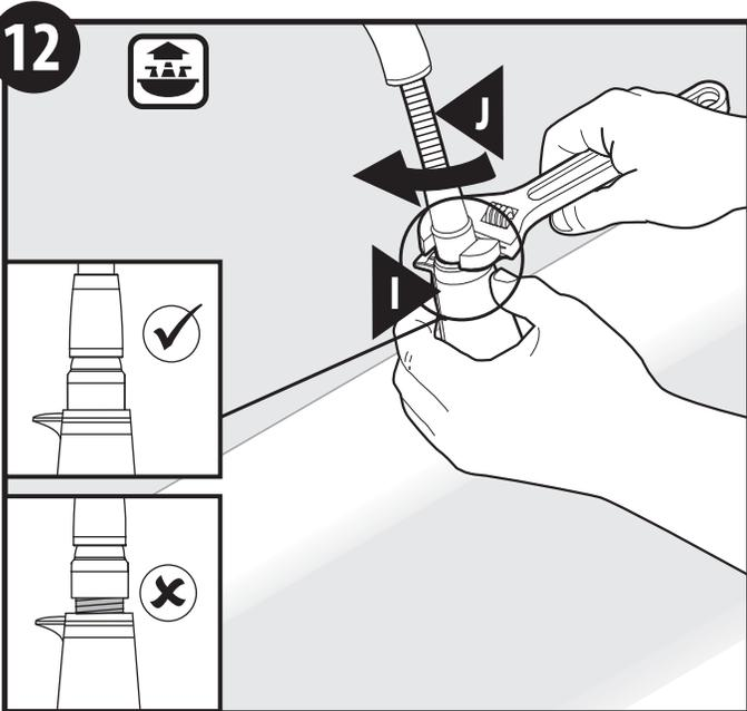
Tighten pulldown hose (J), flush with spray wand (I). Do not overtighten.
