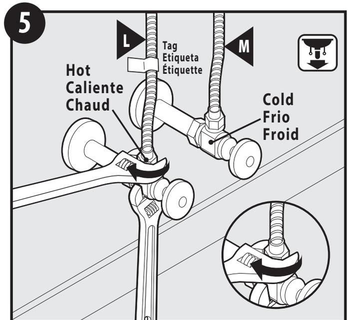
Connect hot (L) and cold (M) supply hoses to water supply valves and tighten with wrench.
