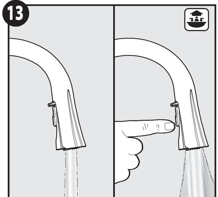
Check operation of spray wand. Turn on faucet, spray wand should be in stream mode. For Kitchen Model S72608: Push and release bottom of button on spray wand. The spray wand should change to spray mode. To switch back to stream mode, push top of button. For Bar S62608 Wand: Push & hold button for spray mode. Release button to return to stream mode.
