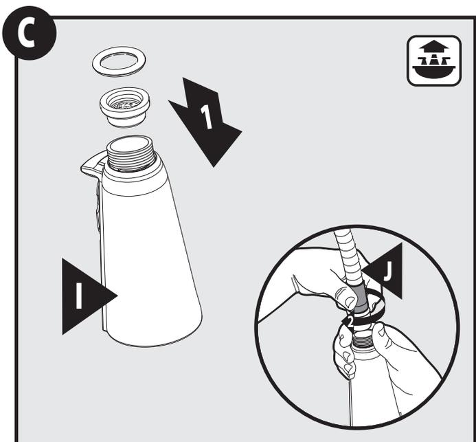
Reinstall screen and o-ring as shown. Thread pull-down hose (J) onto spray wand (I) and tighten as shown in frame 12.
