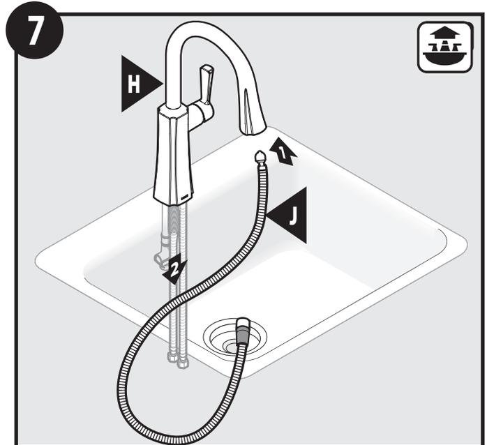
Insert small end of pull-down hose (J) into spout and feed through faucet body (H).
