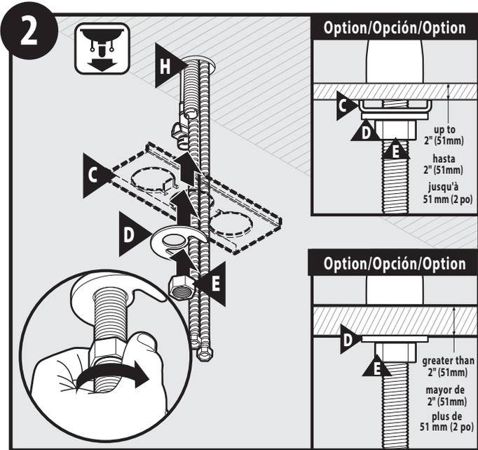
Slide support bracket (C), then mounting washer (D) up onto faucet body (H) under sink and secure with mounting nut (E).
