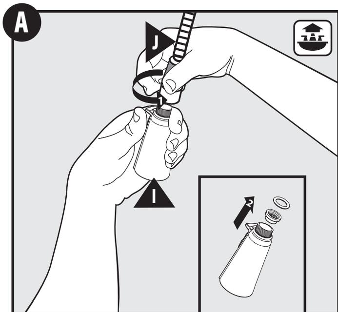
Unscrew pull-down hose (J) from spray wand (I) and remove screen and o-ring.
