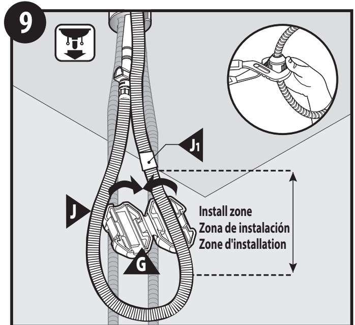
**IMPORTANT** - Locate hose weight locator mark (J1) on pull-down hose (J). Install hose weight (G) just above start of loop curvature in hose on the same side of hose as locator mark.
