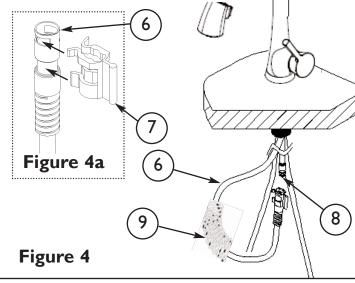
7. Attach CLIP (7) to HOSE (6) as shown. **See Figure 4a**. Connect to valve OUTLET (8) by firmly pressing together until it clicks into place. **See Figure 4**.
