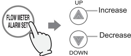
Choose the flow meter alarm setting from the following options: 10 - 60 gallon (40 - 240L) (In 5 gallon (20L) intervals), 70 gallon (260L), 80 gallon (300L), 90 gallon (340L), 100 gallon (380L), 990 gallon.
