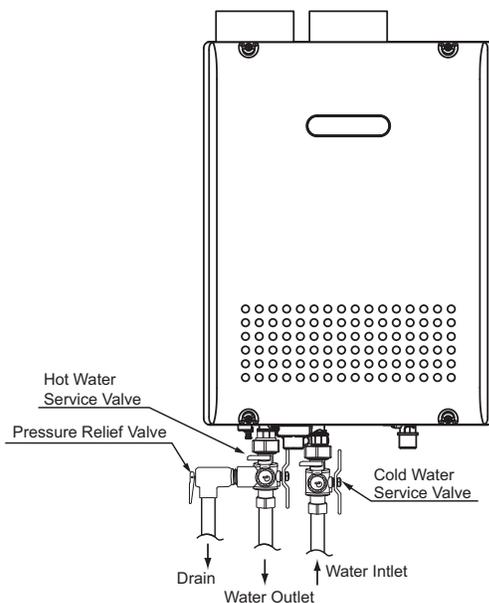
\* Isolation valves may be purchased as an accessory from Noritz. They allow for full diagnostic testing and easy flushing of the system.
