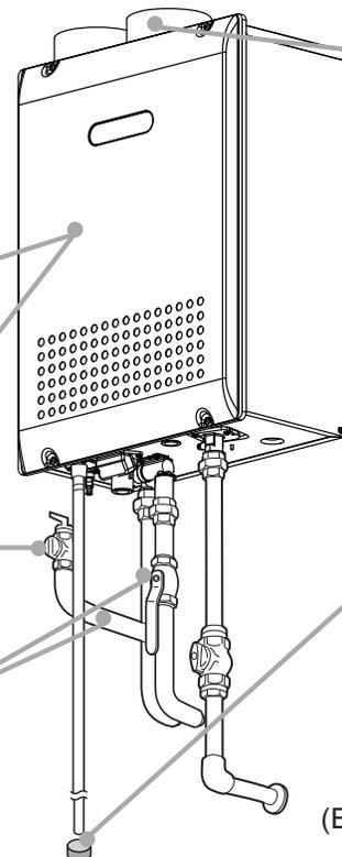
**Check** For dust and soot in the exhaust vent or exhaust vent terminal.
