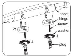
Insert the plugs into the fixing holes of the toilet. Install rubber washer on bottom of hinge. Click the hinges into the seat & cover fixing holes.
