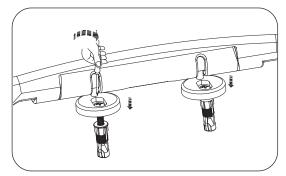
Close the seat and cover onto the toilet and adjust seat and cover to a proper position. Tighten the screws firmly with a screwdriver.
