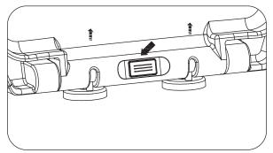
Open the seat and cover. Push the center push button to release seat and cover. Pull upwards the seat and cover to take it off the hinges.
