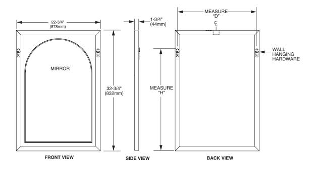
**NOTES:** AFFIX TO A STUD OR PROVIDE ADEQUATE WALL SUPPORT FOR THE SIZE AND WEIGHT OF THE MIRROR.
