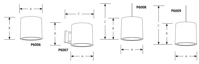
The P6000 Series LED cylinders are nominal 6" cylinders designed to be used with the P8071 series trims. Available in surface, wall, pendant, or cord mount, they provide a cost effective option for LED surface lighting. It is suitable for a wide varity of commercial, retail and institutional applications.
