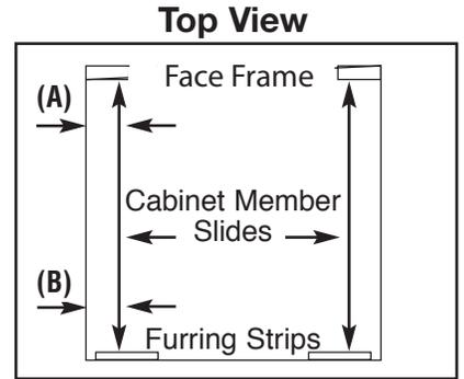
**Step 5:** Mount Rear Bracket. Extend the slide rear mounting bracket until it contacts the rear (Furring Strip). Bottom of slide should be  $1\frac{3}{8}$ " from cabinet floor. Rear mounting bracket should be the same distance from the side cabinet wall at rear of slide as it is up front. Drive mounting screw in center horizontal slot of rear mounting bracket, tighten. Tighten screw in front bracket.
