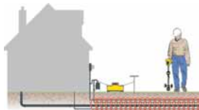
Direct connect to utility lines.
