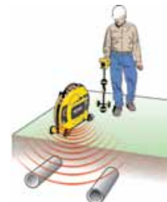
Induce a signal to locate utilities.
