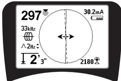
Figure 49 – Screen Display with Distortion Line (Line Trace Mode)
