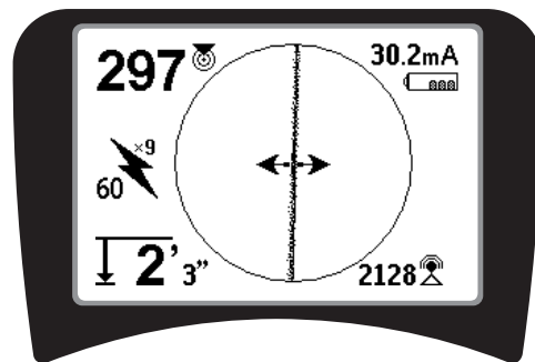
Figure 25 – 60 (9th) Hz Passive Trace Frequency
