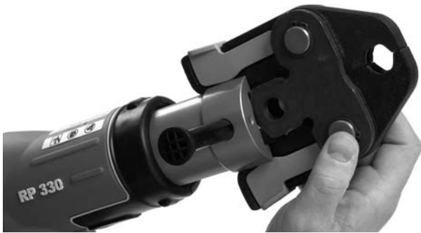
Figure 5 – Slide Attachment Into Tool
