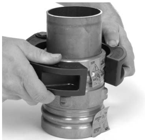
Figure 9 – Installing Press Ring Onto Fitting
