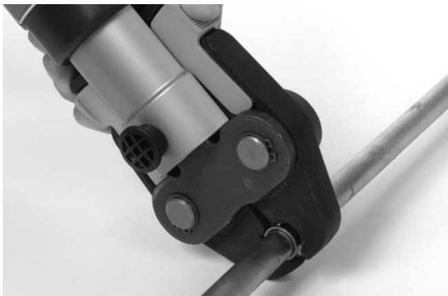
Figure 7 – Placing Scissor-Style Jaw Set Around Fitting
