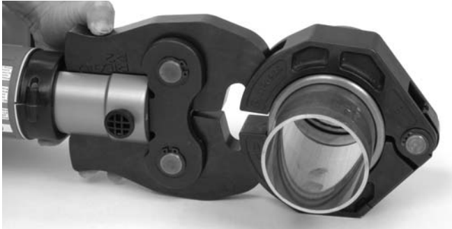
Figure 10 – Attaching Actuator to Press Ring
