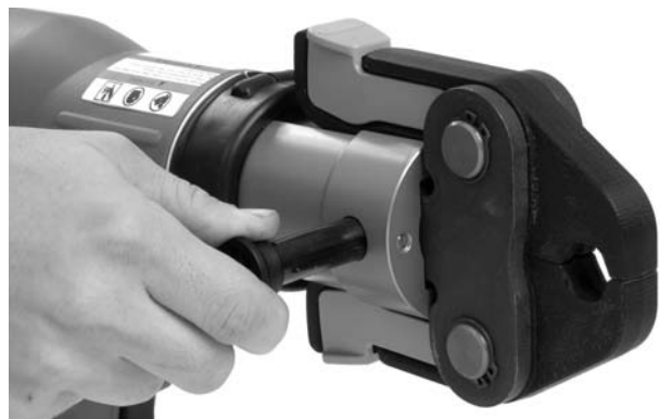
Figure 4 – Fully Open Attachment Mounting Pin
