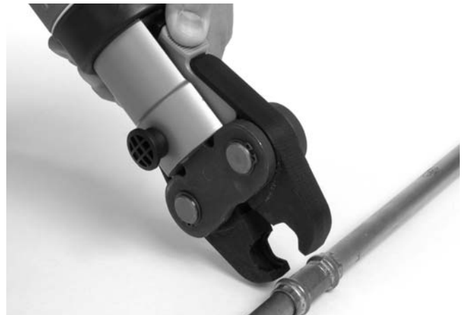
Figure 6 – Opening The Scissor-Style Jaw Set
