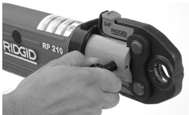
Figure 4 – Fully Open Attachment Mounting Pin
