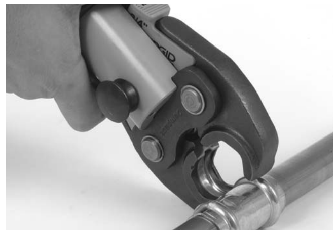
Figure 6 – Opening The Scissor-Style Jaws
