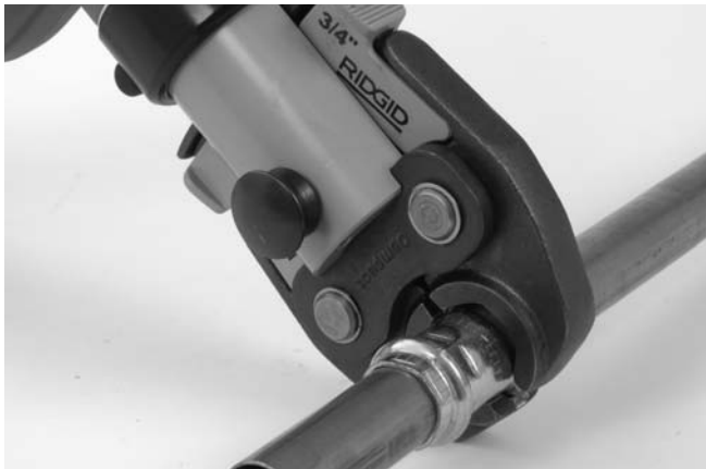
Figure 7 – Placing Scissor-Style Jaw Set Around Fitting
