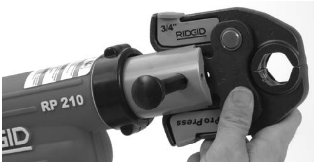
Figure 5 – Slide Attachment Into Tool
