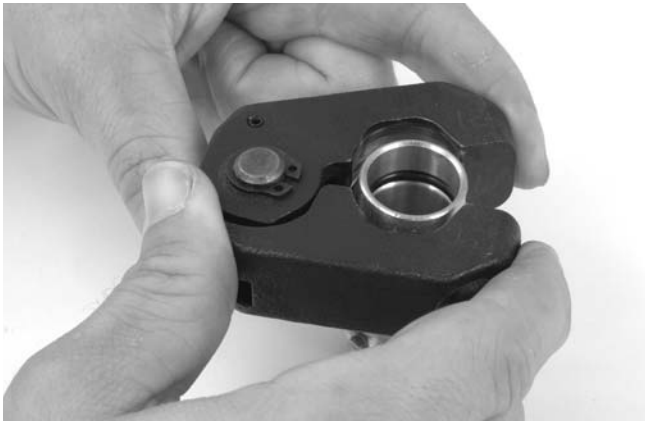
Figure 9 – Installing Press Ring Onto Fitting
