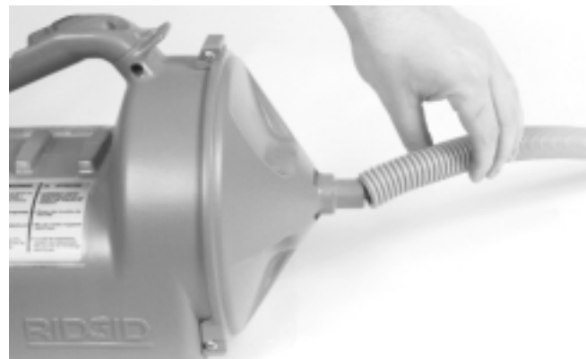
Figure 4 – Attaching Guide Hose to Machine
