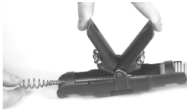
Figure 3 – Feeding Cable Through AUTOFEED™ Assembly
