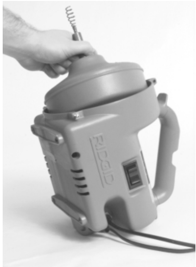
Figure 11 – Inserting Drum Into Machine
