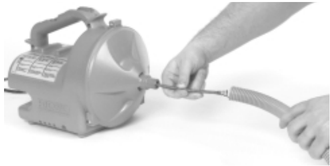
Figure 2 – Feeding Cable into Guide Tube
