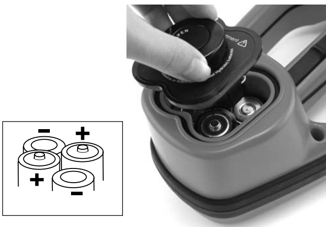
Figure 4 – Compartiment des piles
