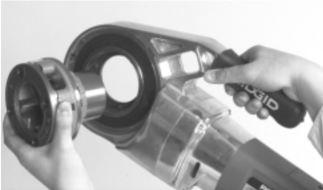
Figure 3 – Installing No. 11-R Die Heads
