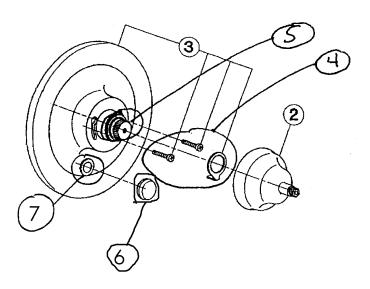
MOUNTING SCREWS+CAM+DIVERTER ASSEMBLY 2303-1210 MOUNTING SCREWS
