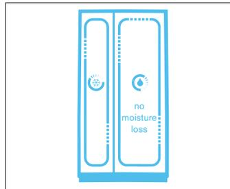
Twin Cooling System® uses two evaporators with only one compressor to independently control the temperature in the refrigerator and freezer.
