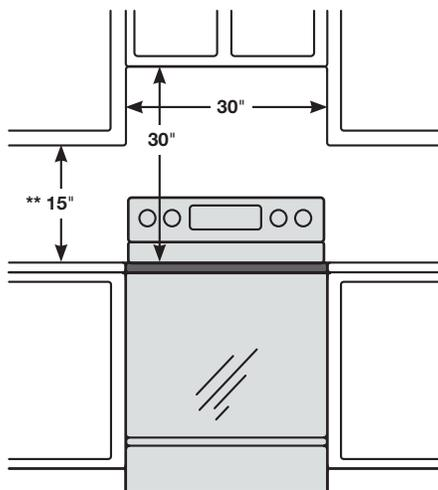
**IMPORTANT:** To eliminate the risk of burns or fire caused by reaching over heated surface units, cabinet storage space located above the surface units should be avoided. If cabinet storage is to be provided, the risk can be reduced by installing a range hood that projects horizontally a minimum of 5" beyond the bottom of the cabinets.
