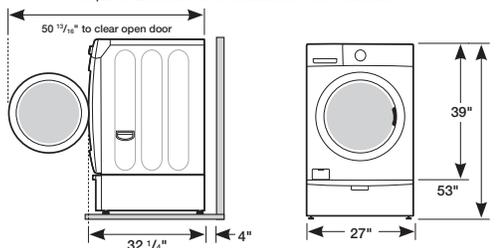
Required Dimensions for Installation With Stacking Kit
