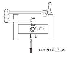
Secure the Pot Filler's flange using the 2 screws provided.
