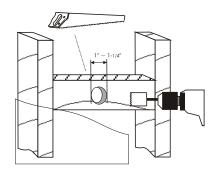
B - If the wall is closed, using a stud finder, mark the location where the flange screws will be fixed onto.
