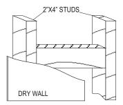
A - In order to assure that the pot filler is firmly secured. It is recommended that the pot filler's flange screws be fixed against wood stud (wood runner/ header).
