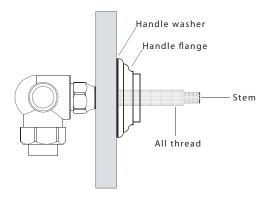
Screw the escutcheon onto the all thread. If there is a gap between the handle flange and the ecsutcheon remove it and cut off the excess thread and stem and re-thread the escutcheon.
