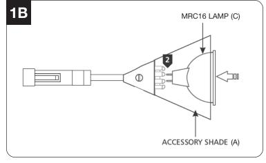
2 Use MAX 50 Watt, MRC16 Halogen Lamp (C). Line up the lamp pins with the socket holes. Insert the MRC16 lamp pins all the wall into the socket holes.
