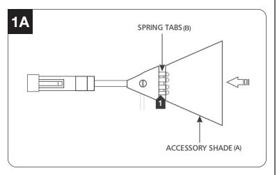
Push the accessory shade (A) (not supplied) all the way onto the spring tabs (B).
