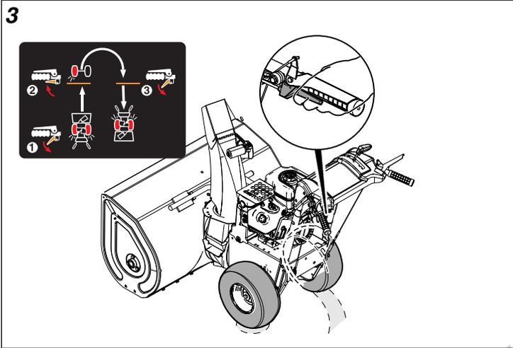
Engaging the Easy Turn traction control lever releases one of the traction wheels, but allows the other wheel to continue driving. Releasing the Easy Turn traction control lever automatically engages both drive wheels for full traction (Figure 4).
