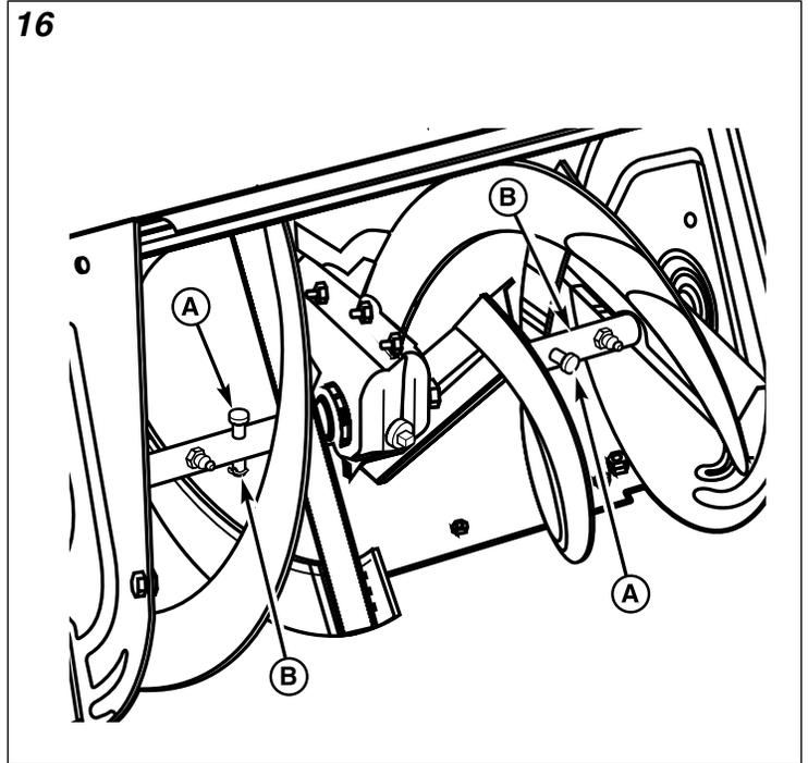
1. Tap out the broken shear pin with a pin punch.
