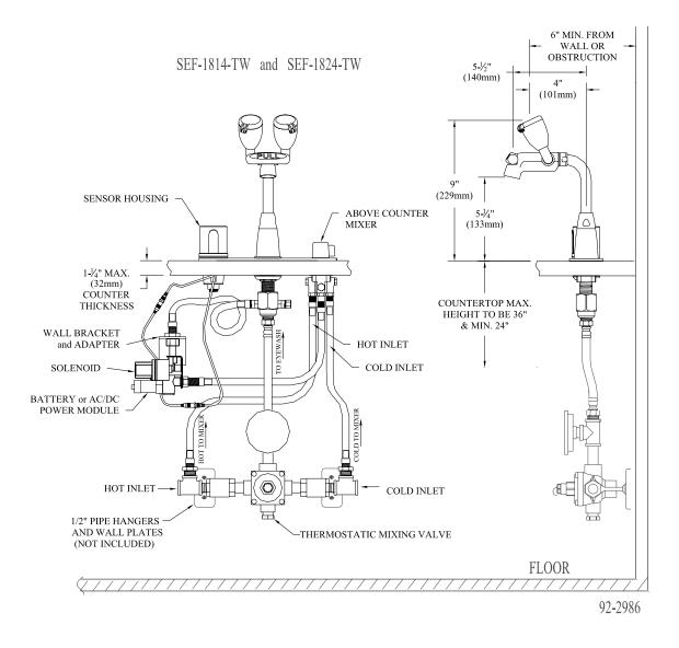
**SEF-1814-TW** -8" Sensorflow, eyewash faucet, ACM, battery and Thermostatic Valve for Eyewash **SEF-1824-TW** -8" Sensorflow, eyewash faucet, ACM, AC/DC and Thermostatic Valve for Eyewash
