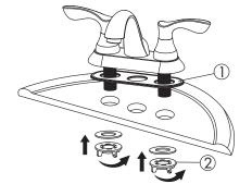
Place the rubber washer (2) to underside of the flange (1). Insert the threaded end of the drain body up through the drain hole and attach flange to the body with the pivot hole (3) pointing to the rear of the sink.
