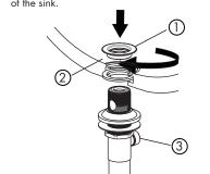
Make connections to water lines. Use 1/2" IPS faucet connections (1), or use 3/8" O.D. ball nose risers (2) with coupling nuts (3). Use wrenches to tighten connections. Take care to not overtighten.
