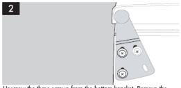
Unscrew the three screws from the bottom bracket. Remove the foot from opposite side.
