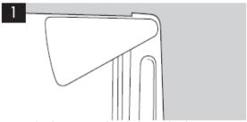
Remove the plastic covering from the bottom door hinge.
