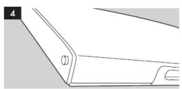
Slide the Table Top Fridge door down about 1.5cm [6"] and off the Top hinge pin and lift away from the Table Top Fridge.
