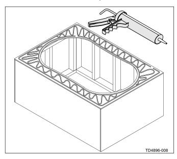
12. Very carefully turn the panel over and place it onto the tub deck. Make sure the panel is correctly positioned. It is important to apply hand pressure to the entire surface of the panel to bond it to the mounting surface and then place weight on top of it to hold it firmly in place.
