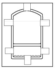
To assist in a secure fit, it is suggested that the Swanstone Recessed Shampoo Shelf be held into place with either masking tape or hot glue. Tape the Recessed Shampoo Shelf into position, or apply a dab of hot glue in each corner. This will hold the Swanstone Recessed Shampoo Shelf in place until the silicone adhesive sets up. It may be necessary to re-caulk the perimeter of the Recessed Shampoo Shelf. Allow 24 hours for drying.
