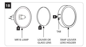
Use **MAX** 50 Watt MR16 Front Cover Halogen Lamp.
