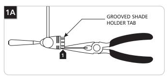
If the Firebird accessory fits tight onto the fixture, then carefully bend the grooved shade holder tabs in slightly with the needlenose pliers. If it fits loose, then carefully bend the grooved shade holder tabs out slightly with the needlenose pliers.
