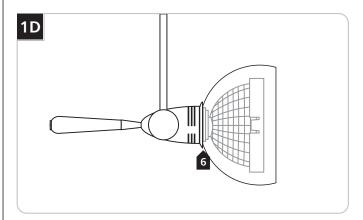
6 Hold the lamp against the glass with the thumb and push the lamp pins all the way into the socket holes; simultaneously push the Firebird accessory metal ring onto the grooved shade holder.
