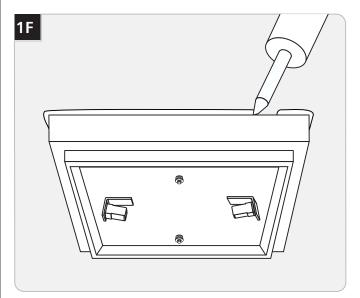
**10** For wet location installation, caulk around the mounting base with waterproof construction sealant.
