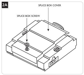
Loosen the center screw on the splice box and remove the cover.
