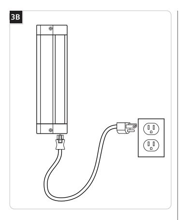
2 Using the Plug-In Wall Feed, plug the Undercabinet unit directly into a wall outlet.
