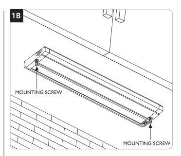
3 Secure the fixture with the provided mounting screws.
