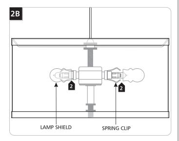
2 Push the lamp shield onto the spring clips
