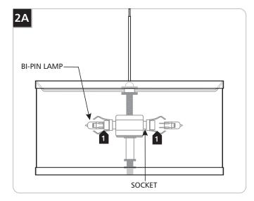
Use **MAX** 35 Watt, Bi-Pin Halogen Lamp With Each Socket.
