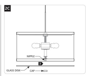
Place the glass disk onto the exposed nipple and secure with the cap. <u>DO NOT OVER TIGHTEN</u> the cap which may cause the glass disk to break.
