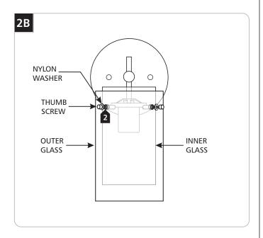
Line up the outer glass holes with the inner glass studs. Secure the outer glass to inner glass with provided three thumb screws and nylon washers.
