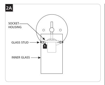
Line up the inner glass holes with the socket housing holes. Tighten the three glass studs completely (through inner glass holes) into the socket housing holes.
