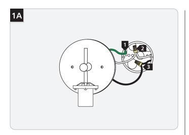
**NOTE:** Use the provided universal round crossbar when the sconce base holes do not line up with the electrical box holes.
