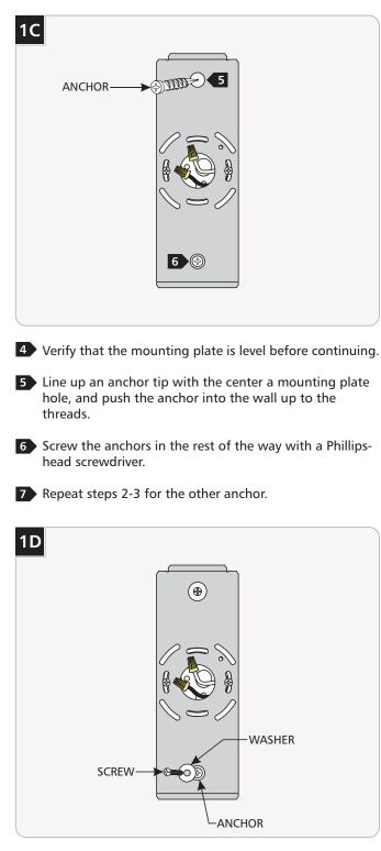
Slide a #8 screw through a washer and screw it into an anchor. Repeat for the other anchor to secure the mounting plate to the wall.
