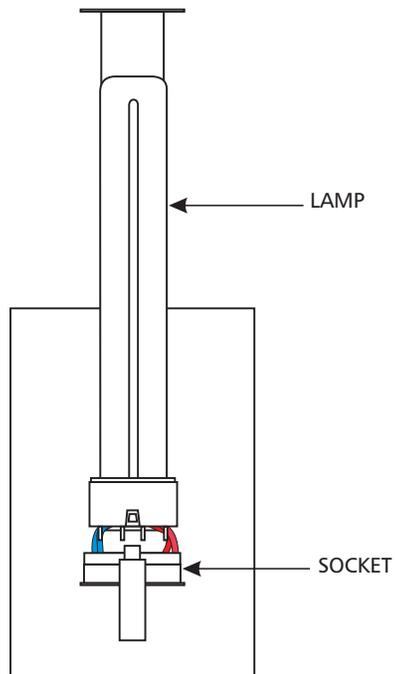
**CAUTION:** To reduce the risk of a burn or electric shock during relamping, disconnect the power to the fixture by turning the wall switch off.
