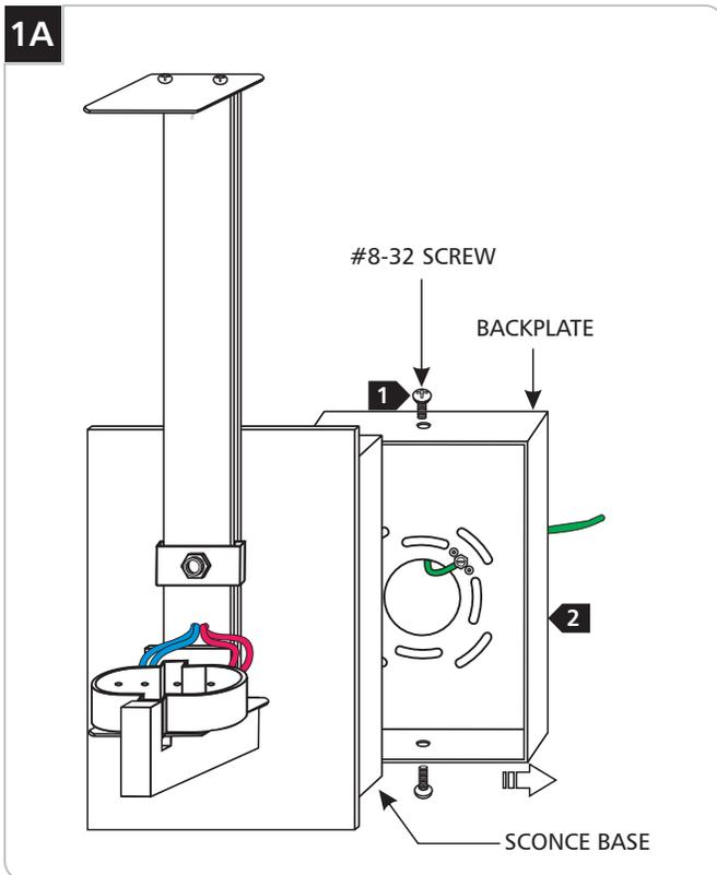
1 Remove the two #8-32 screws on the backplate with a Phillips head screwdriver.
