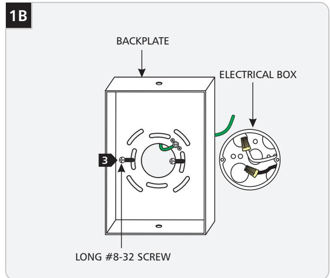
3 Mount the backplate to the electrical box with two long #8-32 screws.
