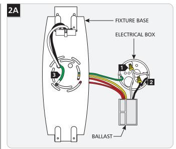
1 Connect the ballast white wire to the neutral power line wire with a wire nut.
