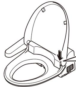
The seat switch is built in here.
