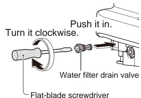
Tighten it securely using a flat-head screwdriver.
