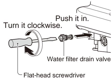
Tighten it securely using a flat-head screwdriver.
