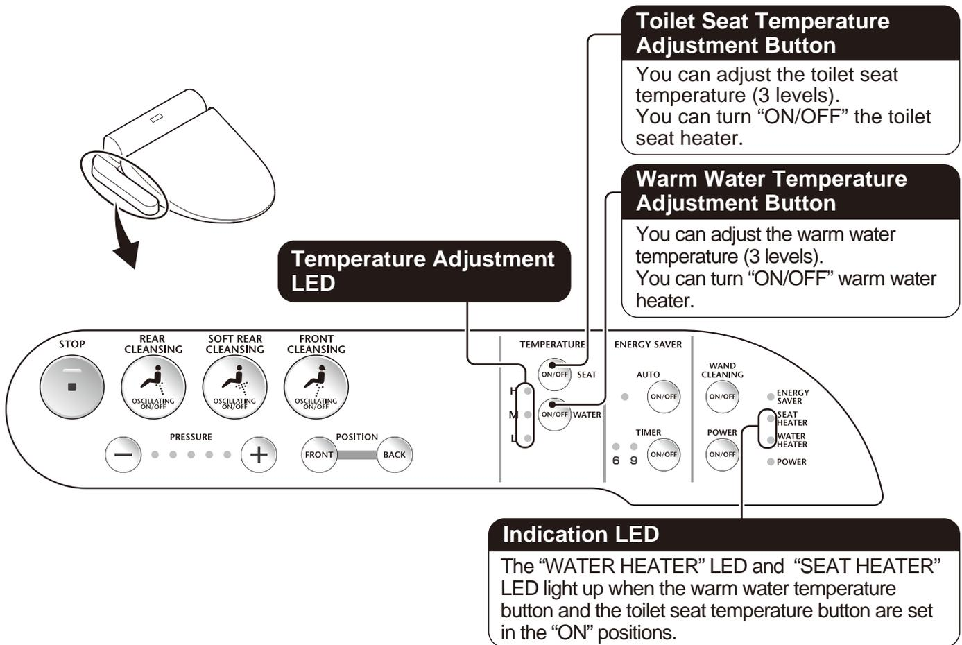
**1** Press the temperature adjustment button(s) on the Washlet control panel.
