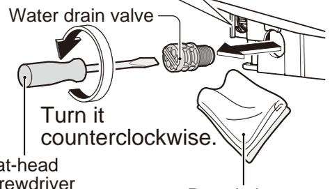
Loosen it by flat-head screwdriver.
