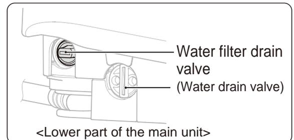
**3** Remove the water filter drain valve.
