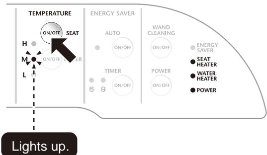
**2** Press the temperature adjustment button repeatedly until the temperature reaches the desired level.
