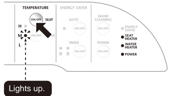
**2** Press the temperature adjustment button repeatedly until the temperature adjustment LED goes out.
