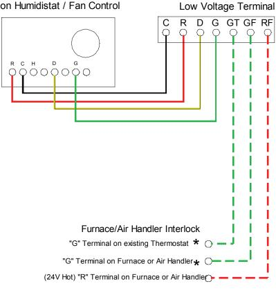
\* Remove Existing Wire Between T-stat "G" and AH/Furnace "G"
