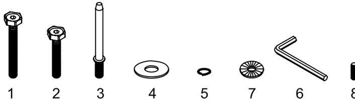
**Step 1.** Put the **Back Frame (A)** on a soft, clean place as shown. Connect the **Seat Box (B)** to the **Back Frame (A)** using the **Flat Washer(4)**, **Spring Washer(5)** and **Long Bolt(1)**. Turn **Long Bolts(1)** with **Wrench(7)** properly. Do not tighten.
