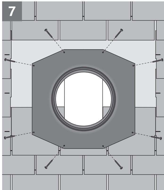
**English:** Center the flashing over the rough opening and secure the flange with the provided  $1\frac{1}{2}$ " (40 mm) screws in all the pre-punched holes along the edges.
