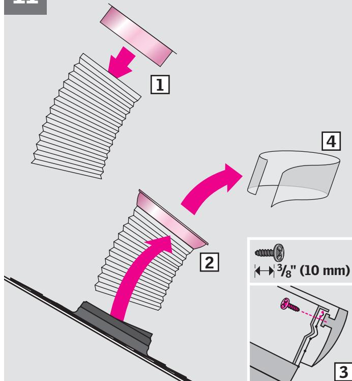
**English:** Press the aluminum ring into the flexible tunnel (1). Install the pivot ring over the aluminum ring and secure it with the  $\frac{3}{8}$ " pan head screws as shown (2, 3). Remove the protective film (4).
