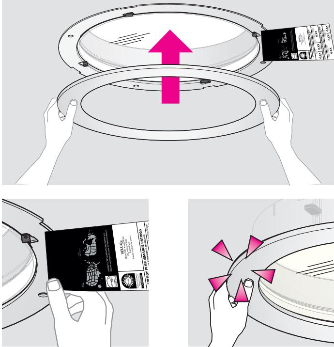
**English:** Install the trim ring by centering under the ceiling ring and snapping the four to six tabs into position. The tabs can also be aligned with the notches and then rotated to secure.
