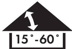
**English:** TGR and TMR are designed for asphalt shingles and wooden shingles up to  $5/16''$  (8 mm) thick and roof pitches between 15-60 °.
