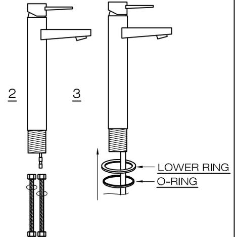
2. CONNECT FLEXIBLE HOSES TO THE BRASS PIPES.
