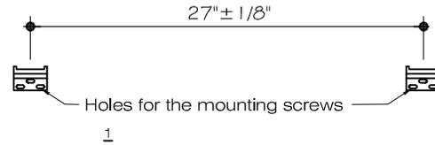
2. Loosen both adjusting screws in the vanity hanging unit. Hang up the vanity to the wall brackets. Tighten adjusting screws.
