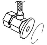
1 SHUT OFF WATER SUPPLY. REMOVE OLD FAUCET AND FLEXIBLE HOSES. CLEAN SINK SURFACE IN PREPARATION FOR THE NEW FAUCET.
