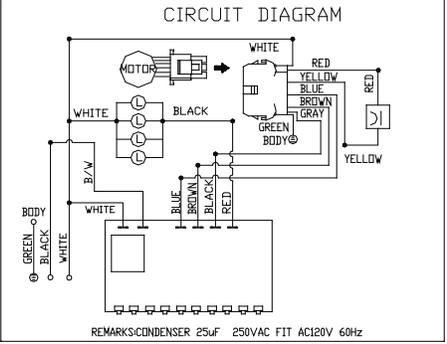
REMARKS:CONDENSER 25uF 250VAC FIT AC120V 60Hz
