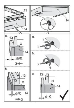
If the shelf (13) and drawer (14) are not aligned at the front (d≠0), first completely pull out the drawer to access the drawer opening mechanism on the back wall. Press on the spacer (A) to release the mechanism. Rotate the spacer to adjust the length.
