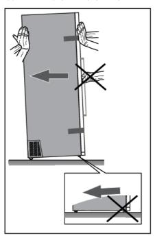
When moving the appliance, be careful not to push it on the floor because of potential damages. There are two casters on the back of the appliance housing, that make moving the appliance around easier.
