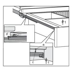
The drawer can also be removed from the appliance without removing the serving bottle shelf from its rails. To do this, fully open the drawer, lift it at the front (1) and pull it towards you.
