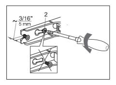
Partly (by no more than 5 mm) undo the hinge screws (2) at the top and bottom.
