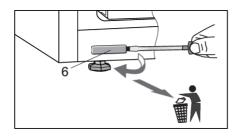
7. Remove the cap (6) and discard into the bin for plastic waste.
