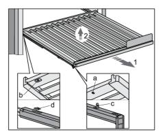
To remove a shelf from the appliance, fully extend the telescopic rails (1), and then vertically lift the shelf (2) to remove it from the rails. Take care not to damage the door gasket.
