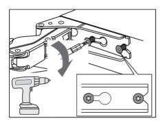
Tighten the screws. The screws should be tightened to a torque of 4.5 lb/ft (6.2 Nm).
