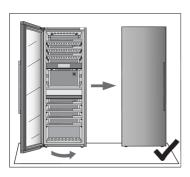
15. Close the door and make sure it is aligned with the housing. The housing side and the edge of the door should be parallel.
