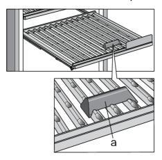
The wooden bottle shelf with moon shaped recesses allows you to load the bottles onto the shelf cross-wise.
